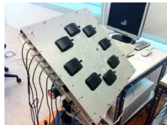
Figure 4 GNSS smart antenna proof-of-concept prototype.
