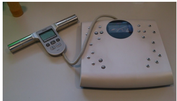
Figure 3. Modified bathroom scale for the acquisition of ECG (leads I, II and III), IPG and BCG
